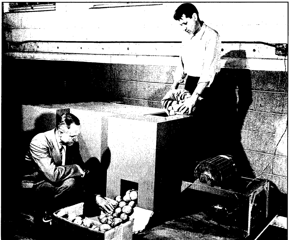
Potatoes being irradiated during a food preservation study. This process did not cause the food itself to become radioactive. Rather, it destroyed organisms which would have caused spoilage of the food. This process lengthened the storage life of these foods.
